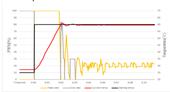
Fig. 5. The Fuzzy Q-learning PID Controller for the Temperature of 60 Degrees Response
