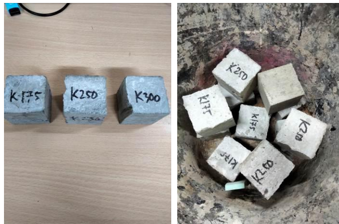
Figure 3: Manufacture of water absorption test sample completed within conditioning
